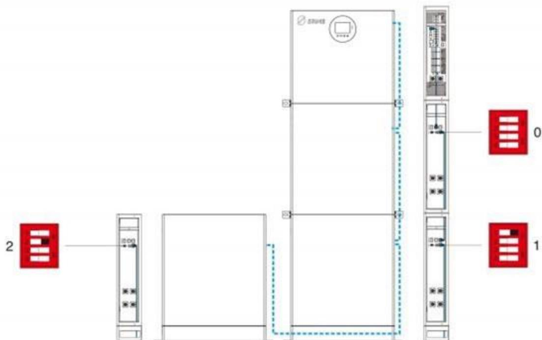
20kwh Wiring diagram:
