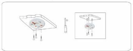
Step7:Fix the cover into the lamp and end the installation.
