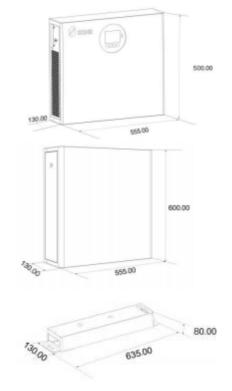
Inverter dimensions (L\*W\*H) :555\*130\*500mm Battery dimensions (L\*W\*H) :555\*130\*600mm Base dimensions (L\*W\*H) :635\*130\*80mm
