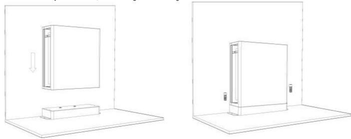
Install the second battery in the same way. After the installation is complete, install the wall fixing bracket.
